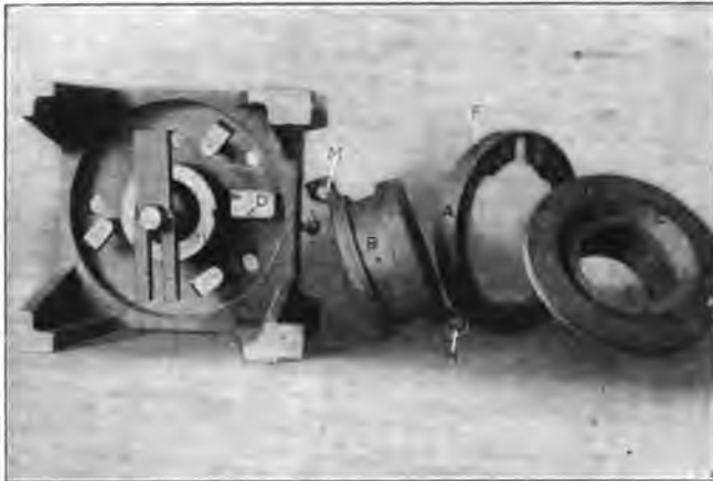
Fig. 16. Drill Jig for Parts of Friction Clutches shown at the Right
